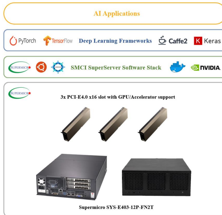
Figure 1 - AI/ML Software Stack
