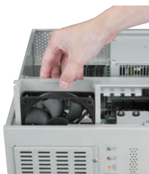
Easy-to-maintain cooling fan
